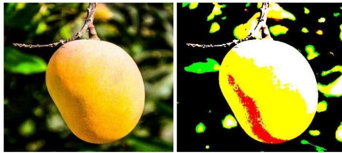
Figure 4. Effect of Image Normalization. Input image (left) and normalized output image (right) Normalization rescales pixel values to a consistent range, reducing brightness variation and improving contrast for more stable model training.
