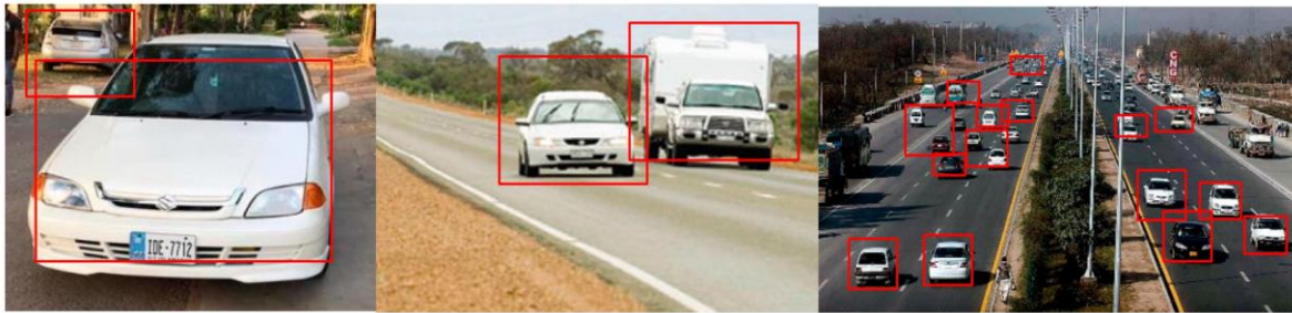
Figure 1. Examples of vehicle detection from traffic in Pakistan.
