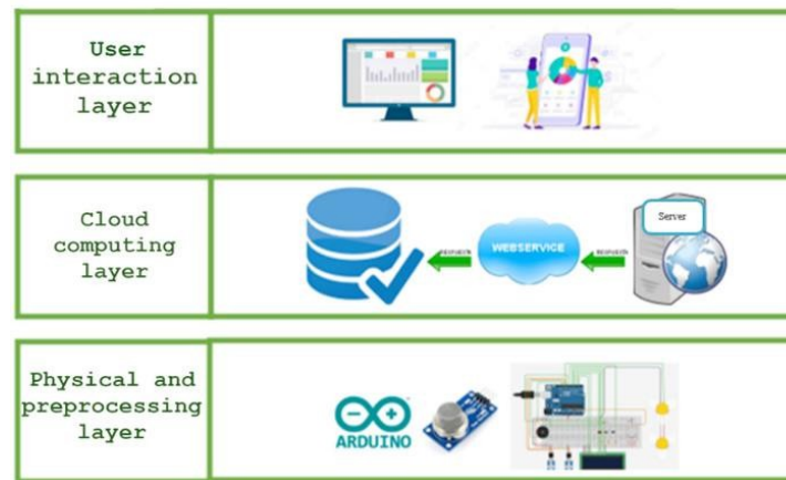
Figure 2. Air Quality Monitoring System Architecture
