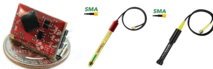
Figure 2. Embedded system, Lab Oxygen Probe & Lab Grade pH Probe IoT devices for measuring water quality.
