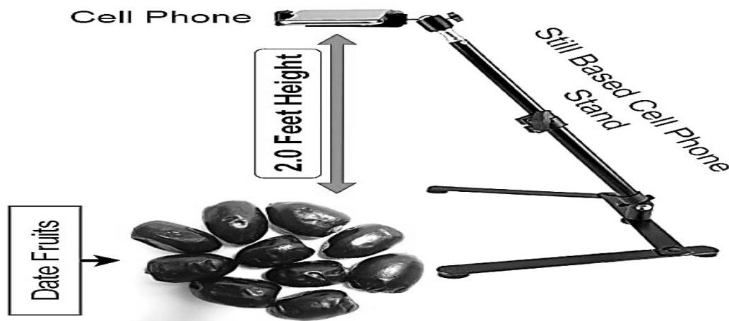
Figure 1: Setup of Image Capturing
