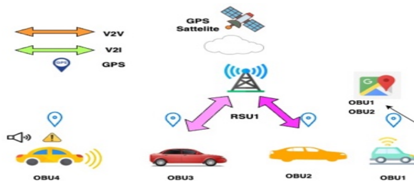
Figure 1. Internet of Automobile architecture showing various components for improved security.
