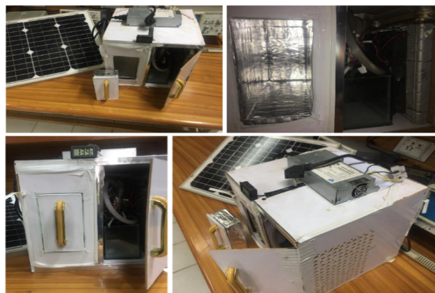
Figure.3. Final Product of Peltier-Based Thermoelectric Cooling Module
