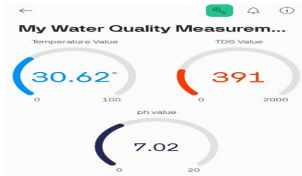
Figure 3. Water quality Blynk IOT application where sensors collected data shows in gauge forms
