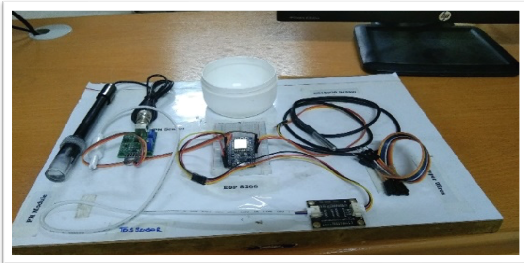
Figure 1. Hardware part of water quality through sensors
