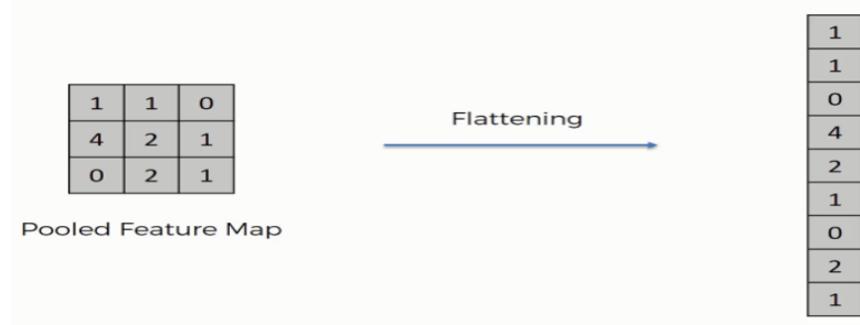
Figure 7. Working principle of flatten layer.
